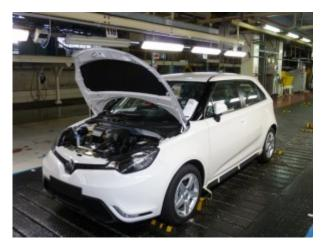
With the front exterior panelwork added, the car is almost ready for final checking to be carried out.
