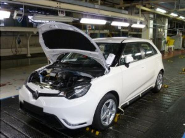
With the front exterior panelwork added, the car is almost ready for final checking to be carried out.
