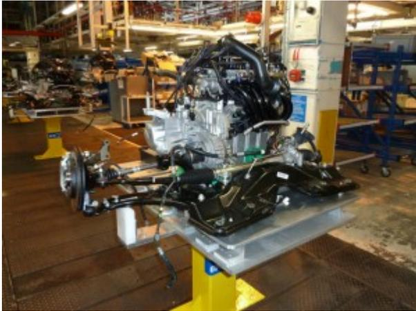
When the front sub-frame, steering rack, hubs, driveshafts and brake discs/calipers are added, the assembly looks like this.
