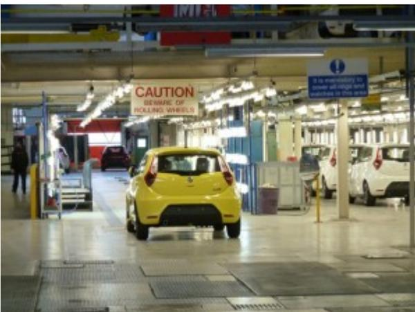
The completed cars are rolled along towards the test areas by means of a 'moving floor' system.
