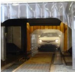
Here a new MG3 is seen as it is about to emerge from the 'Storm Test' chamber, in which each completed car is sprayed with water at high pressure.
