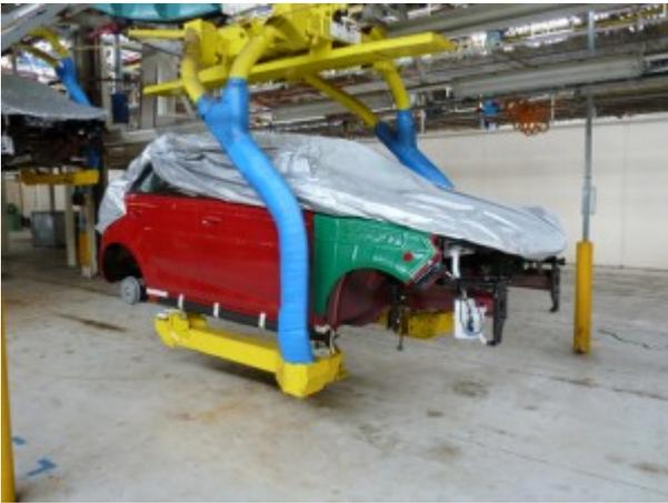
When the part-completed body shells arrive from China at the Longbridge factory, they look like this (MG3 shown here), awaiting front end components.
