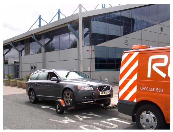
The 'Rapid Deployable Trailer' has transformed the way in which RAC patrols work, enabling vehicles to be recovered by a patrol if they can't be fixed at the roadside.
