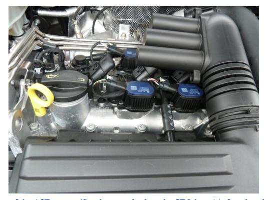
The heart of the ACT system (fitted as standard on the GT I drove) is found at the top of the engine and linked to camshaft operation. When the ACT system comes into play, the two centre cylinders are effectively shut down, thus saving fuel.
