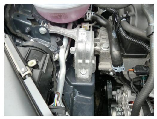
The engine mounting set-up is now standardised across the Golf range, helping to make significant savings in production costs.
