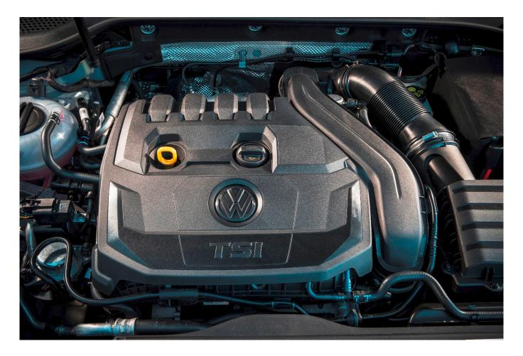
For the VW Golf range the new 1.5 EVO engine is available in two states of tune, 130 and 150 hp. Both are turbocharged four cylinder petrol engines and are available with six-speed
