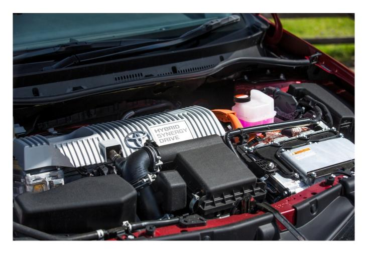
The Toyota Hybrid Synergy Drive system's 1.8 litre VVT-i petrol engine and electric motor together generate maximum power of 134 hp, giving the Auris Hybrid hatchback a 0–62mph acceleration time of 10.9 seconds and a top speed of 112mph. In common with all other Toyota models the Auris hybrid is covered by a five-year/100,000 mile warranty.
