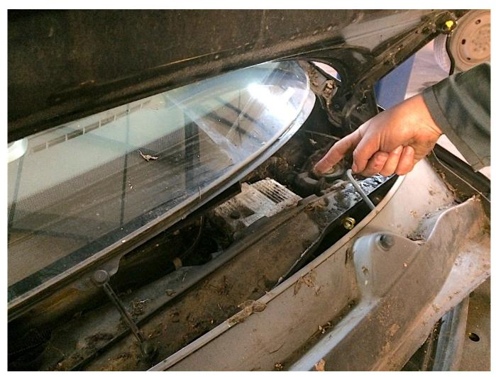
For reasons unknown, Vauxhall chose to locate this 2009 Corsa's Electronic Control Unit (ECU) immediately beneath the scuttle, where it can so easily become waterlogged...
