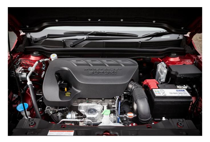
The 1.0 litre three cylinder direct injection turbocharged Boosterjet petrol engine delivers 111 hp with 170 Nm (125 lb.ft) of torque from 2,000rpm. It offers 9% more torque than the outgoing 1.6 litre non-turbo petrol unit, with 11% lower CO2 emissions and 10% better Combined Cycle fuel economy.
