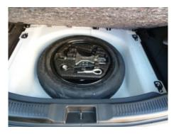
The 'space saver' spare wheel lives in its own well pressed into the car's structure, beneath the floor of the boot.
