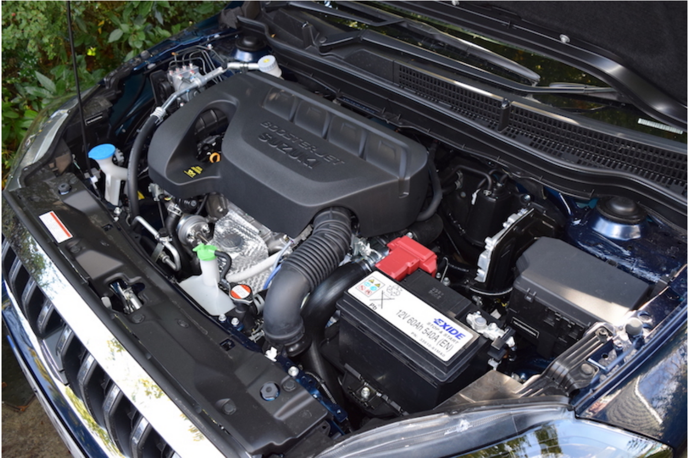
The four cylinder, 16 valve 1.4 litre Boosterjet K14C petrol motor in our test car.
