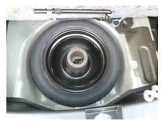
The 'space saver' spare wheel lives in its own compartment beneath the main floor of the boot.
