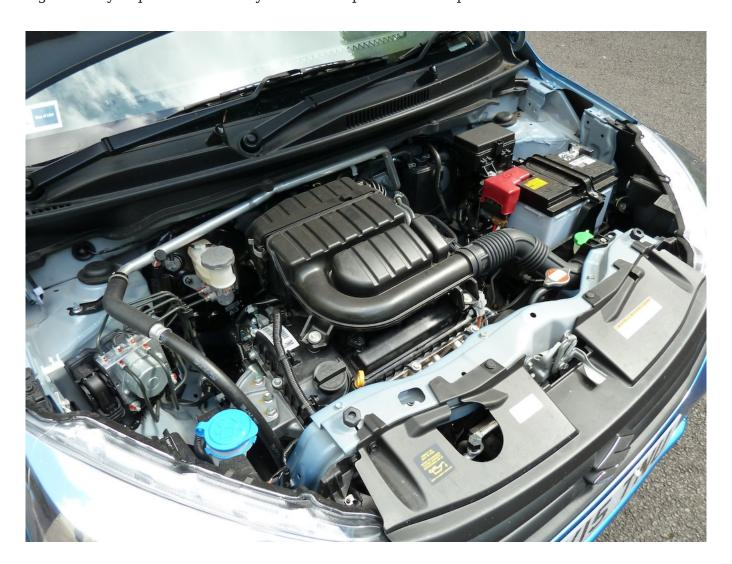
This engine features a higher compression ratio (12.0:1 compared with the K10B's 11.0:1) and provides greater thermal efficiency. It also incorporates friction reduction technology, including roller-rocker type valve lifters (with variable valve timing too).
