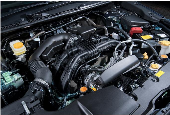
For the new model range the 2.0 litre 147 hp diesel engine – quite understandably, due to the fall in oil-burner sales – has been dropped from the range to be replaced by a new 1.6 litre 114 hp normally-aspirated port injection four cylinder 'Boxer' unit. By far the best selling engine will be Subaru's 2.0 litre, 150 hp flat-four 'Boxer' horizontally-opposed direct injection non-turbo petrol unit.
