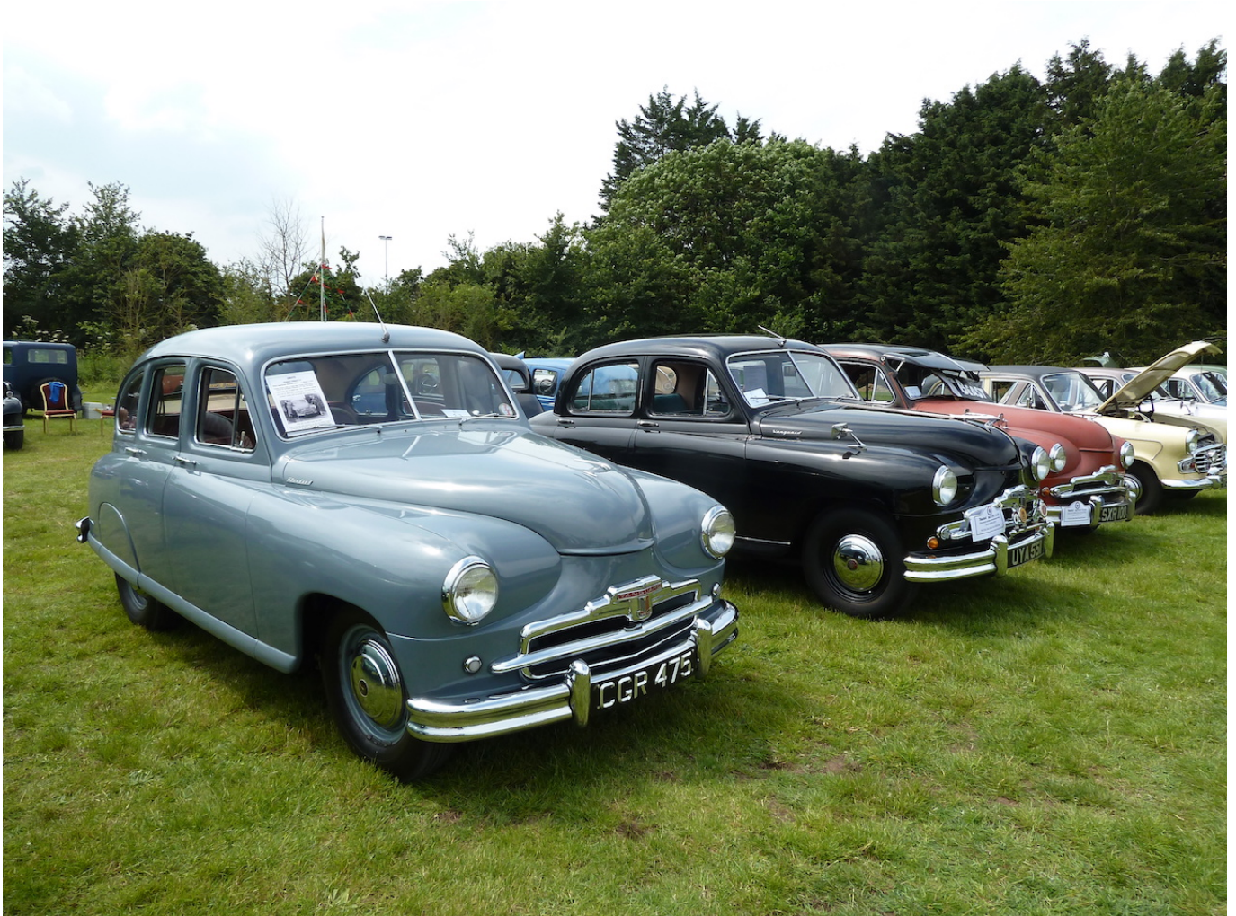
On the left in this shot is Mark Denton's Phase IA salon, showing the three bar grille style of these models, also the rear wheel covers (fitted to Phase I models from late 1949, and Phase IAs). The black car is a Phase II, with 'notchback' rear bodywork.
