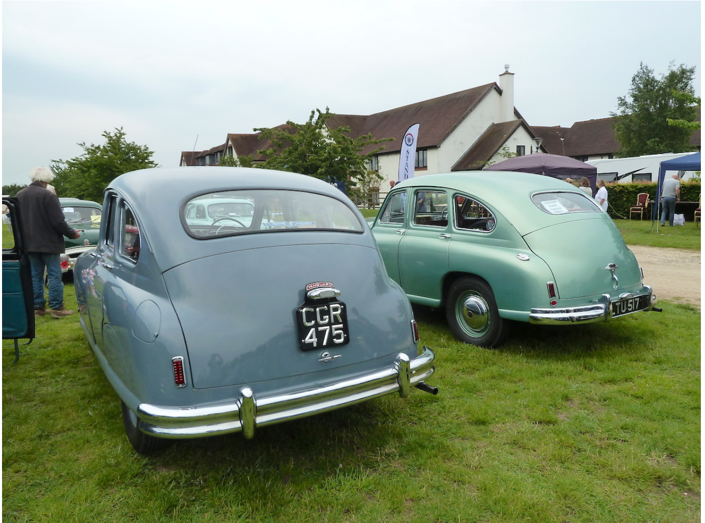
Rear end contrast between the Phase I (on the right in this shot) and the Phase IA, with its larger rear window.
