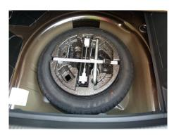
Each of the Spacebacks I sampled had a steel 'temporary' space-saving spare wheel (a £75 option) housed within the well beneath the boot floor.
