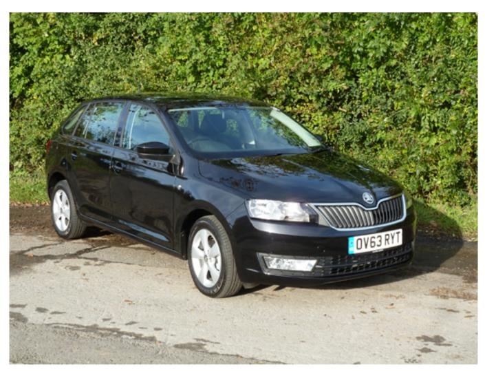
Wrap-around lamps are visible from the sides as well as from the front of the car.
