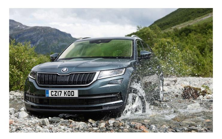
The Kodiaq is 4,697 mm (15.41 ft) in length, 1,882 mm (6.17 ft) wide and 1,676 mm (5.50 ft) high so it is visually a substantial looking heavyweight SUV. With its short front and rear overhangs and long 2,790 mm (9.15 ft) wheelbase it looks purposeful and capable as an on/off roader, even though it uses the same platform as the highly praised Skoda Superb saloons and estates.
