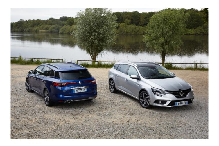
Mechanically the same as the immensely popular Mégane Hatchback, the Sport Tourer offers a basic boot space with a low load floor of 521 litres (18.40 cu.ft), but folding away the off-set split rear three seats gradually increases this to 1,504 litres (53.11 cu.ft).
