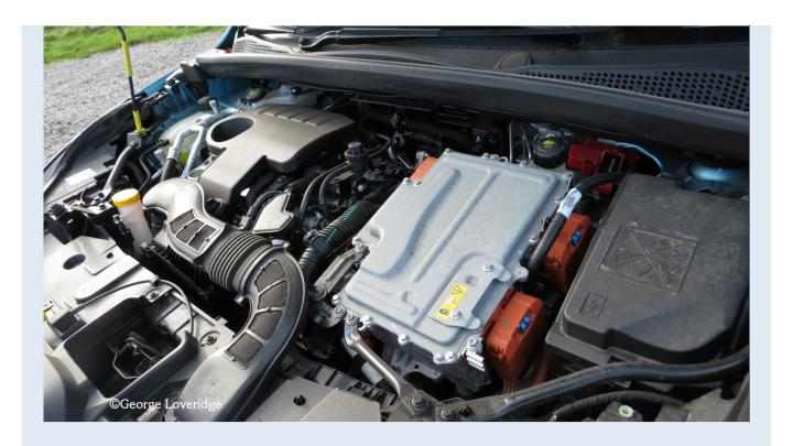
Power: 142 hp at 5,600 rpm, 160 hp combined with the electric motors.
