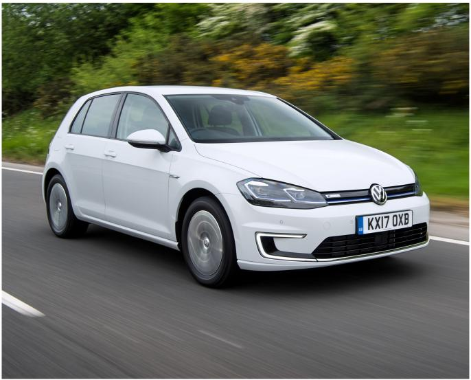
The battery can be charged to 80% capacity within 45 minutes at a DC CCS charging station (40kW). When charged overnight or during the work day from a wallbox (AC, 7.2kW), the battery is ready to go again with 100% capacity in less than six hours. The e-Golf can also be charged in around 17 hours via a standard, domestic three-pin UK plug (AC, 2.3kW).
