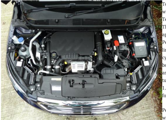
Hidden beneath the covers is a three cylinder, 1.2 litre petrol engine developing 110 bhp and providing very willing performance.
