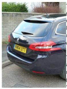
The tailgate opens from bumper-level, aiding the loading and unloading of heavy/large items. The rear lamp units run around the rear corners of the car.
