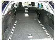
Especially helpful is the ultra-rapid 'one touch' folding arrangement for the rear seat backs, instantly converting the car to van-like load-carrying mode.
