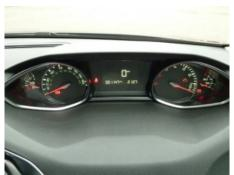
Instrumentation is positioned higher than is usually the case, just below the windscreen, and an unmistakable digital readout of the speed is also incorporated.
