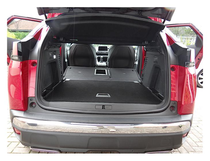
The luggage area can be enlarged by dropping down flat the rear seats (60/40 split) to extend this to a maximum of 1,670 litres (58.97 cu.ft), and there is more storage space under the boot floor around the space saver spare wheel.
