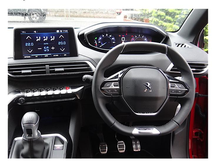
Placing the main digital vehicle read-out information (speed, revs, fuel and temperatures plus operational graphics) high up and straight ahead of the driver means there is no need for the person in control to take their eyes far from the road at any time.
