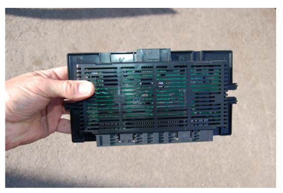
This shot shows the control unit for a number of systems on a BMW (just a few years old). One of its functions is to activate the reversing lamps, and failure of this part of the unit meant a hefty bill for the car's owner.
