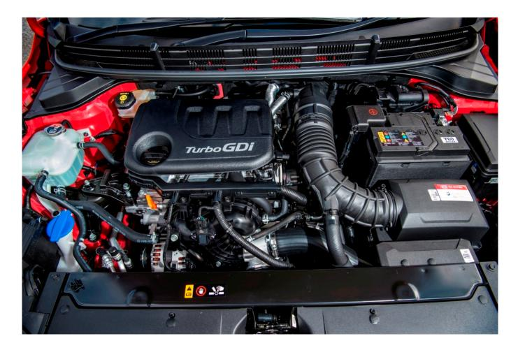
The 1.0 litre three-cylinder T-GDi turbo petrol engine is a bright and lively performer although much more vocal than some other units in this sector. There was a prominent growl under acceleration and some more sound deadening between the engine bay and the passenger compartment could be needed. Once cruising speeds had been reached the noise intrusion died away. It was just another point that added to the lack of refinement that most of its competitor models provide.
