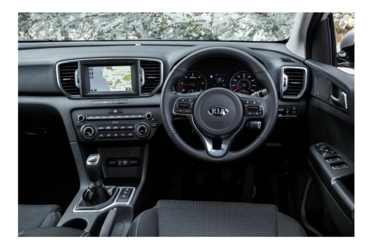
Overall body height is the same but the floor is lower by 40 mm (1.6 in) for easier access and you sit lower, although still with a high-riding feel. Narrower front and rear screen pillars have improved vision at oblique junctions. A generally comfortable cabin is pleasantly furnished, although some colour combinations look better than others. Door pockets are slim but there's a large central cubby box for storage.
