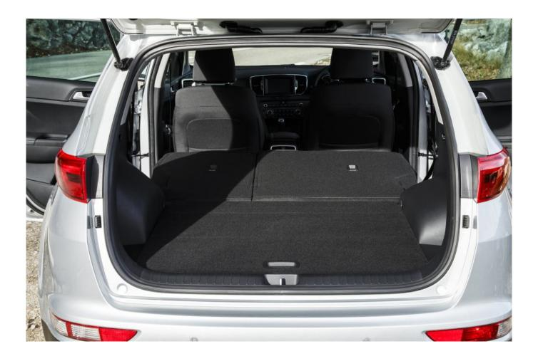
The boot is exceptionally wide, even between the intruding wheel arches. Cargo volume with all seats in use is up by 26 litres (0.92 cu.ft) to 491 (17.3 cu.ft), expandable to 1,480 litres (52.3 cu.ft) with the rear setbacks folded. In length the floor extends, according to our tape, to almost 1.5 metres (4 ft 11 in), still with an upward slope but half as steep as in the previous Sportage, points out Luke Ayres, Kia's Sportage product specialist.
