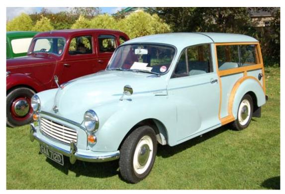
The distinctive Traveller estates provide more luggage space than the saloons. The woodwork is an integral part of the body structure and MUST be sound!
