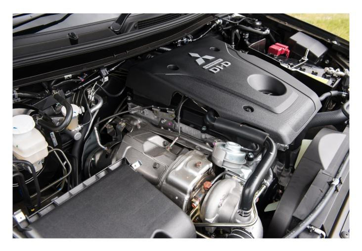
The well-proven 2.4 litre turbodiesel engine is strong thanks to the 430 Nm (317 lb.ft) of torque. It can sound a bit agricultural on start-up but essentially it is a commercial vehicle so it lacks some of the refinement in the powertrain department compared to an SUV.
