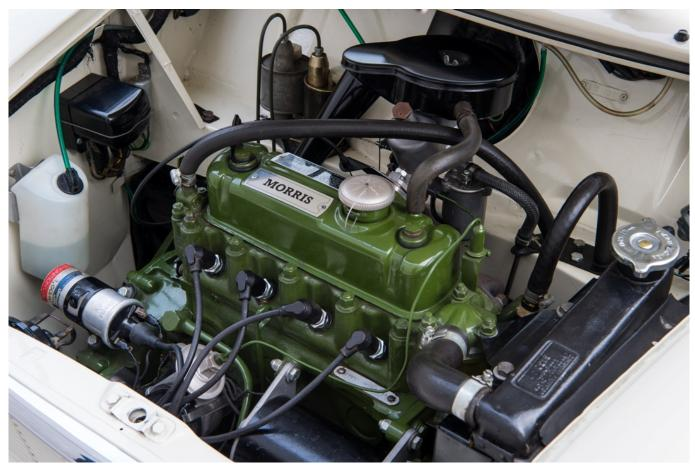
The BMC Mini's 848cc A Series engine was developed from the 948cc unit of the Austin A35, but in the front wheel drive Mini was installed transversely on top of the gearbox. For its time this motor provided sprightly performance, excellent fuel economy (around 45 to 50 mpg) and was reliable.
