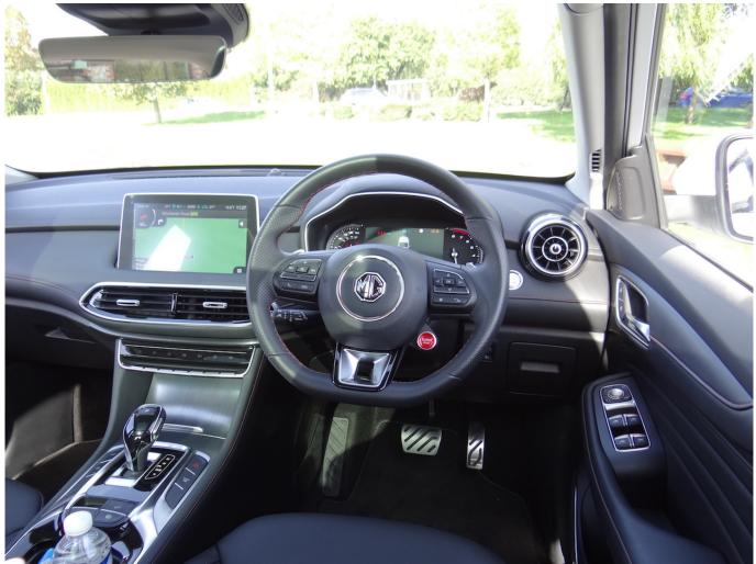
The same goes for the curious digital instrument display behind the reach and rake adjustable steering wheel.
