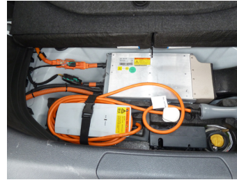
The charging apparatus is stored in its own compartment beneath the normal boot's floor, at the back of the vehicle.
