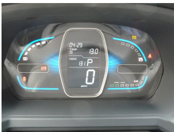
The instrument panel is easy to assimilate and informs the driver of whether the car is using power or is in 'regeneration' mode.
