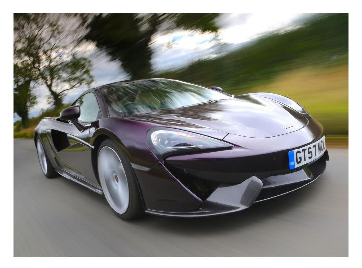
The 570GT shares its carbon-fibre MonoCell chassis and tub with the 540C coupé and 570S coupé as members of their Sports Series. For the first time McLaren use 'superformed' aluminium body panels allowing for a more complex design, they say. It maintains the
