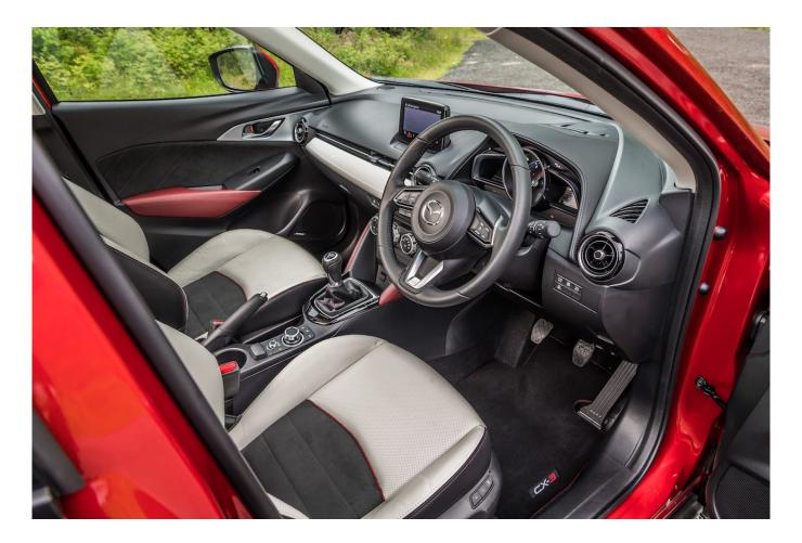
There's a seven-inch multi-media colour touch screen on the dash and a circular controller placed to hand behind the conventional gear lever. It works with compatible internet-enabled Apple and Android smartphones. So-called MZD-Connect also supports iPod, MP3 and CD playback, plus SMS and email readout functions.
