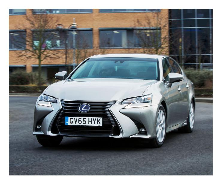
The GS 450h has a 3.5 litre V6 288 bhp petrol engine and a compact 197 bhp water-cooled electric motor, producing a top speed of 155 mph and zero to 62 mph takes 5.9 seconds. The Combined Cycle fuel consumption is 46.3 mpg with 141 g/km of CO2 emissions so VED road tax costs £190 First Year rate and then £130 thereafter with Benefit-in-Kind tax rated as 27%.
