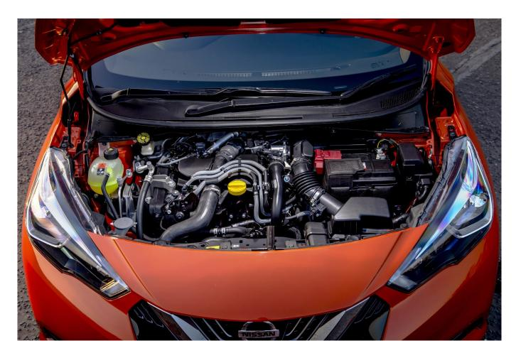
The 898 cc turbo three-pot petrol unit produces 90 hp and 150 Nm (111 lb.ft) of torque but
