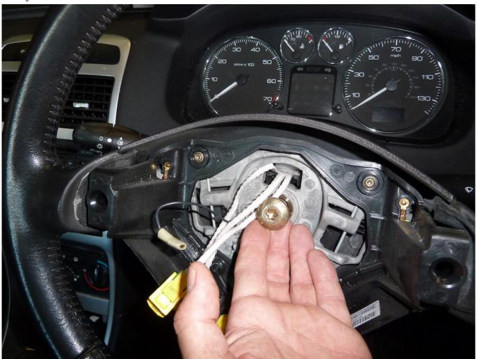
Leave the wheel's securing nut/bolt/screw in place, partially loosened, when attempting to remove the wheel.
