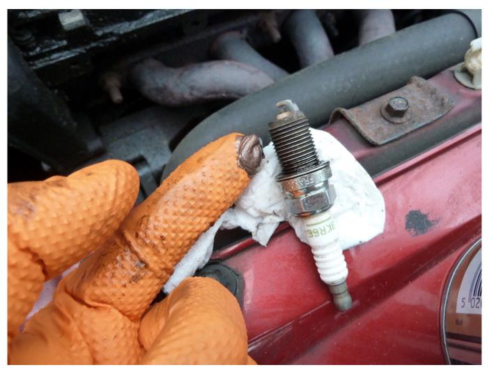
The application of a little copper-based anti-seize grease on re-installation will help prevent the plugs from seizing, aiding removal in the future.
