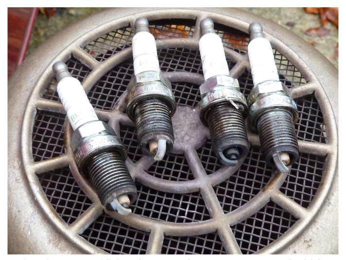
These plugs were carefully heated on a garage heater on a 'warm' setting; this did the trick!
