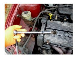
Use a quality spark plug spanner with a rubber insert that firmly grips the plug; essential when they live in deep wells...
