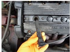
Take great care when detaching the high tension connector and lead from each spark plug; a special tool may be needed.
