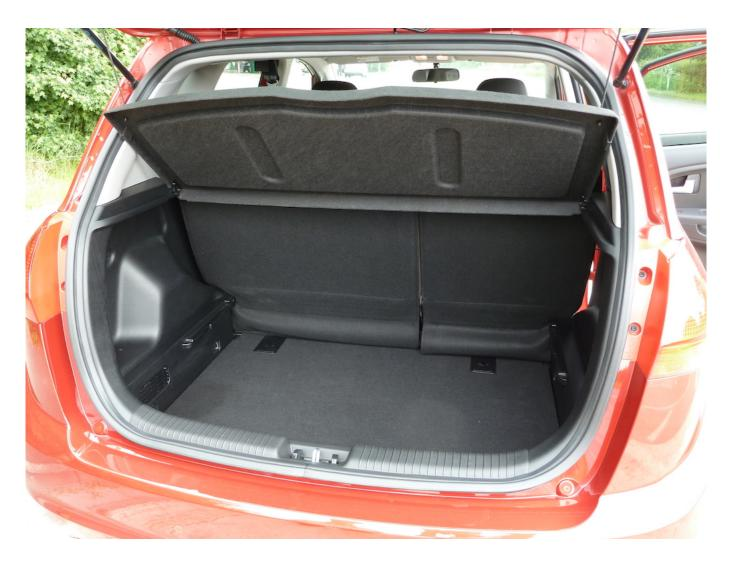
To effectively turn the Venga into a 'small van' when required, the rear seats incorporate another useful trick, in the form of a 'Fold and Dive' function which allows them to sink into the car's floor, then providing a completely flat load floor and a total capacity of 1,253 litres (44.25 cu.ft).
