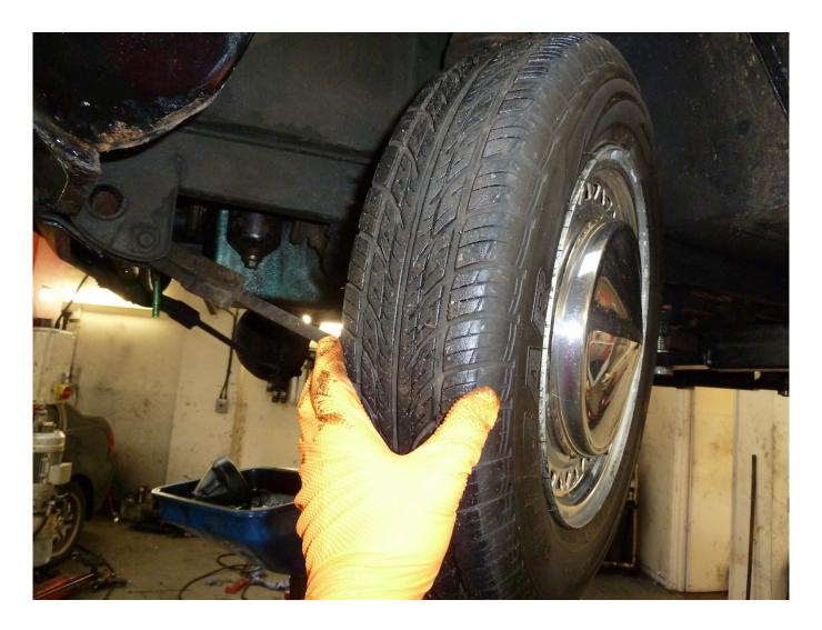
If the vehicle has not been used for a long while, carefully check the condition of the treads and sidewalls before you take it out again.
