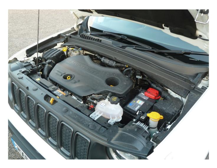
Alternative engines offered in the Renegade line-up include 1.0 litre three cylinder and 1.3 litre four cylinder turbocharged units, and an updated 1.6 litre MultiJet-II diesel (as well as the 2.0 litre version, as tested). The diesel engines incorporate Selective Catalytic Reduction (SCR) technology.
