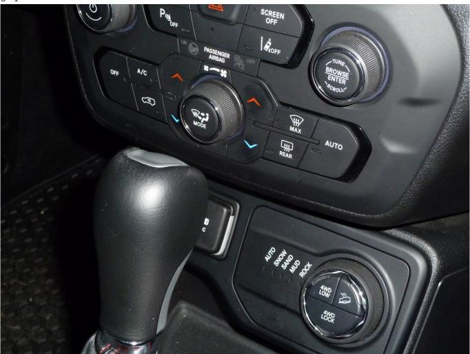
The 'Jeep Active' four wheel drive system operates automatically (with no driver intervention) and is designed to seamlessly switch into and out of all wheel drive mode at any normal road speed, as required and according to road conditions. It is also said to 'deliver yaw correction during dynamic events' and improves both understeer and oversteer situations.
