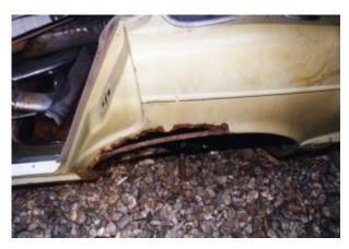
Detailed assessment is advised of the wheel arch lips (which can disintegrate), the sills, the lower edges of the doors, and the rear wing bottoms.
