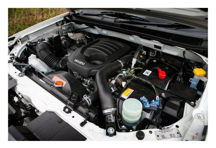
Under the big bonnet there is a comparatively small sub-2.0 litre turbodiesel four cylinder engine which works hard to perform and lets you know when heading towards maximum revs and it becomes boomy. Matched to a smooth six-speed auto-box the performance is adequate but not head-turning, but its overdrive higher ratios help it ease past 30 mpg overall. Use the box and that figure will dramatically fall away.
