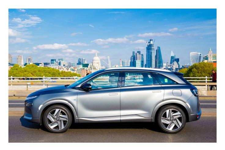
The bespoke platform for the Nexo carries three hydrogen fuel tanks giving a range of over 400 miles when the gas is passed over a very compact stack of fuel cells and electricity flows to the electric motor pushing out the equivalent of over 160 hp to the front wheels.
