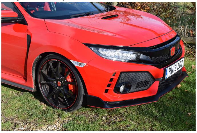
Race-inspired features of the current models include the brake cooling vents (to cool the large and effective Brembo discs and calipers), aerodynamic rear spoiler/wing, vented aluminium bonnet and centrally-positioned triple exhaust outlets.
