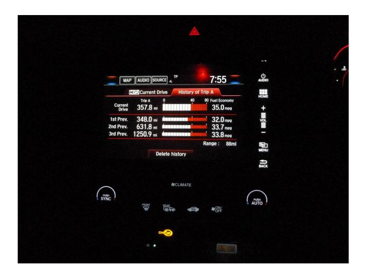
As with other models in the company's range, and as mentioned earlier, Honda's on-board computer system screen display can be set to show previous average fuel consumption figures, obtained between re-sets of the twin 'trip meter' mileage recorders. (The figures recorded previously by other drivers of my test car had apparently varied between 32.0 and 33.8 mpg).
