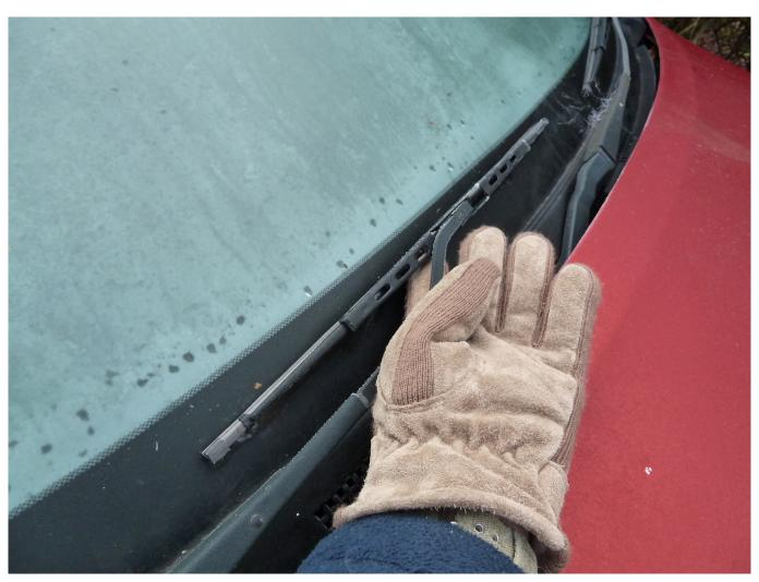
Carefully lift your screen wipers away from the iced-up glass BEFORE turning on the wipers... see text.
