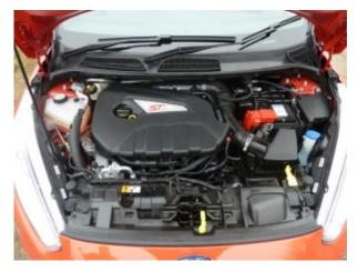
The engine bay is tightly packed; the willing 182 PS 1.6 litre turbocharged EcoBoost motor is produced at Ford's Bridgend plant.
