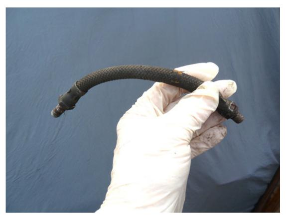
This flexible hose from a hydraulically activated clutch system looked fine from the outside, but was almost completely choked within, due to disintegration of the internal walls. This resulted in severe clutch slip after every gearchange, due to the fluid being unable to move rapidly back through the hose to the master cylinder and its fluid reservoir
