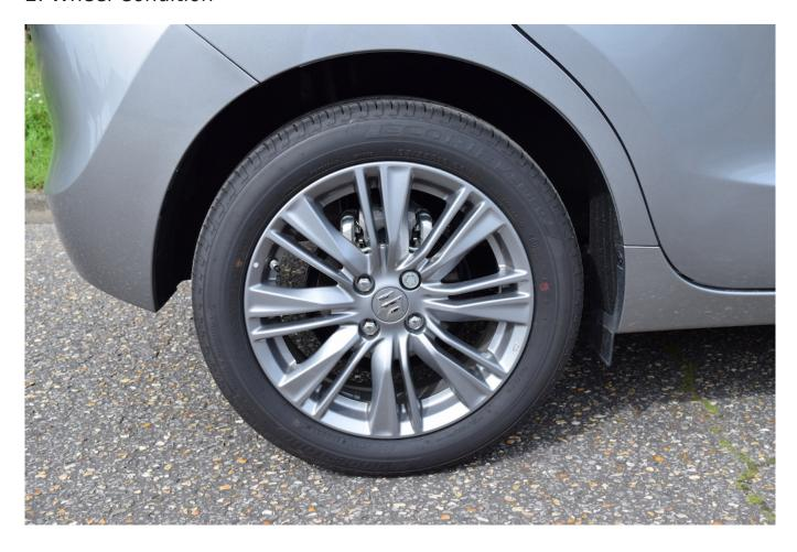
A well-driven car may look good on paper, but the wheels may have had some significant wear. Fortunately, this is something that's easy to see on inspection. You can easily check the hub and wheel for any scratches or irregularities – as well as the wheel bearings (with the car safely supported and the wheel clear of the ground, movement in the bearings can be felt while the wheel is 'rocked' by hand, and if the wheel is rotated by hand, resulting 'grumbling' noises indicate wear).
