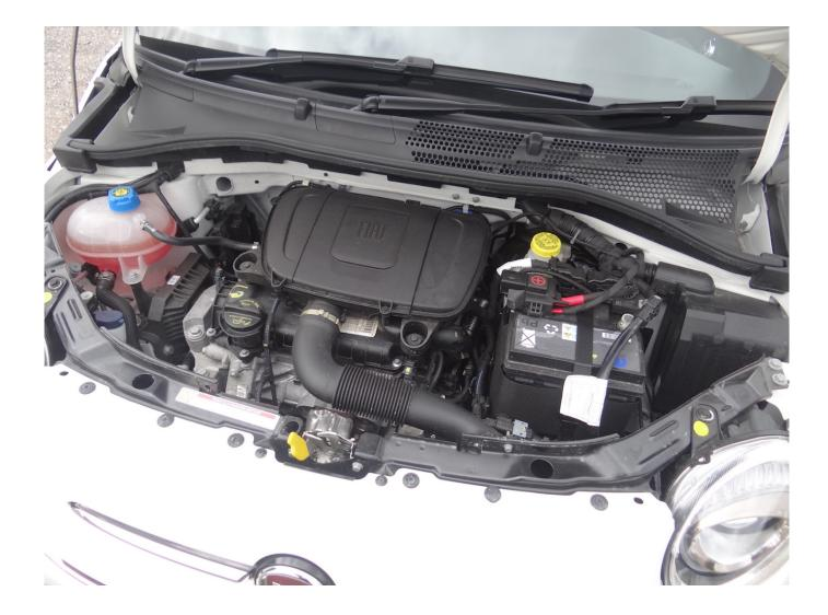
The BSG system is mounted directly onto the engine and is operated by the belt that also drives the auxiliaries. It recovers energy during braking and deceleration, stores it in a small lithium battery with a capacity of 11Ah, and uses it, at a maximum power of 3,600 W, to restart the engine in Stop & Start mode and to assist it during acceleration.
