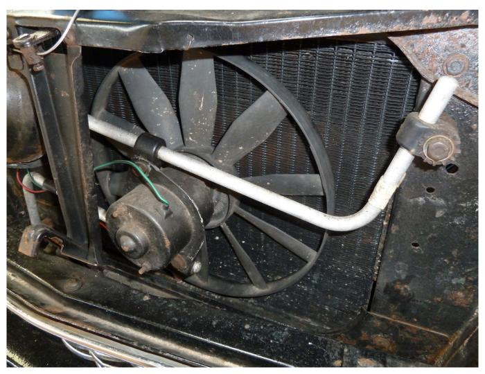
Fitting an extra, thermostatically-controlled, electrically-operated fan helps to keep underbonnet temperatures as low as possible...
