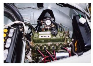
Enginuity. Under the bonnet of the A35 is a four cylinder overhead valve motor, providing willing performance and good fuel economy.
